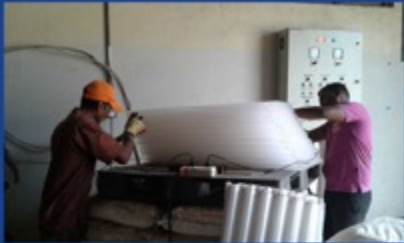
TUBE DECK ASSEMBLING
