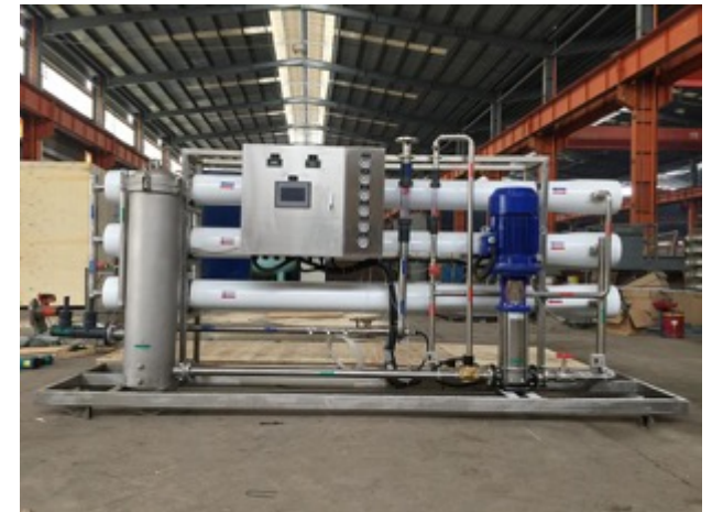
RO desalination systems
