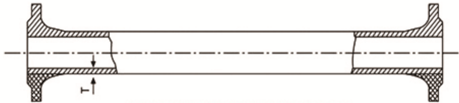
pipes with integrally cast flanges
