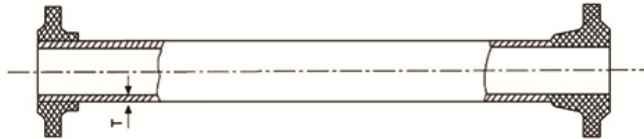
pipes with screwd-on or weld-on flanges
