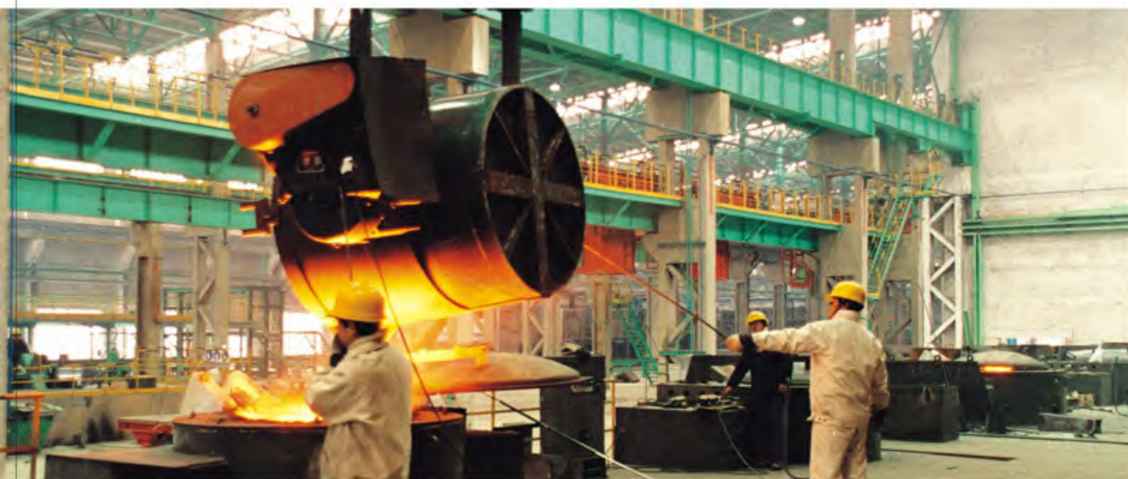
电炉升温及调质 Heating and spheroidization in induction furnace
